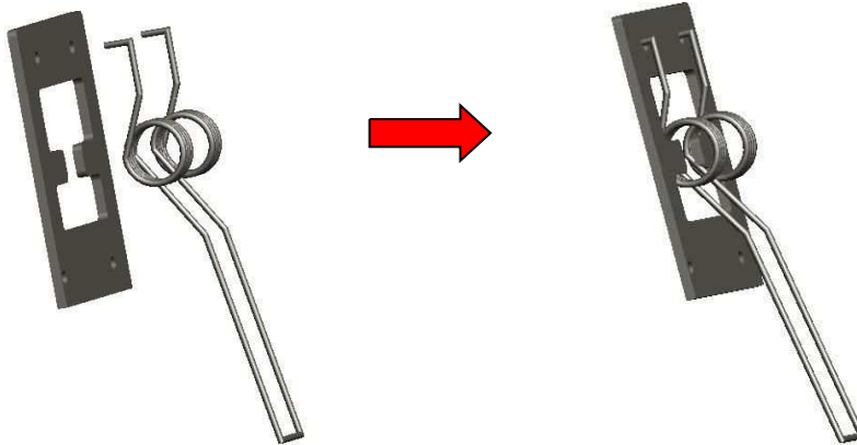
Step1. Attach the spring to bracket
